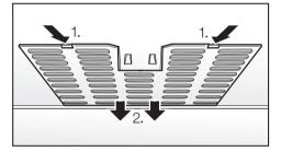
Unhook the filter cover, 1. in each side of the drawer and remove them along with the filter mat downwards starting from 2.
